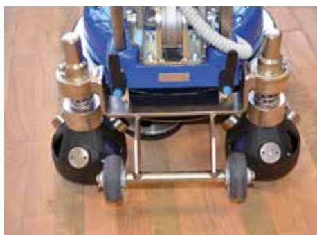
New spherical wheels reinforced and singularly damped.
